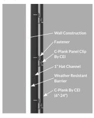
3" C-Plank Panel Clip (.75 clips per ft<sup>2</sup>)
