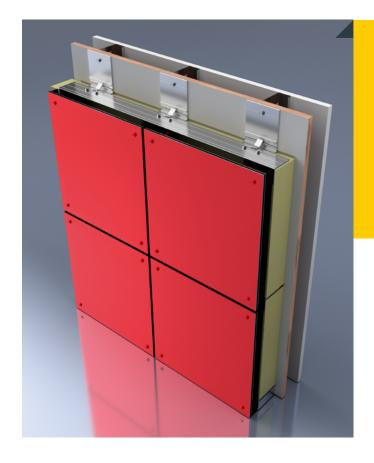
CEI Materials' E1000 panel system is easily installed to a wide variety of substrates and sub girt systems. The system can be provided in HPL, Aluminum Plate and MCM. Flat panels have exposed fasteners and install rapidly reducing installation costs. Panel sizes vary and are designed in conjunction with one another based off shop drawings, field measurements or finished panel sizes provided by client.
